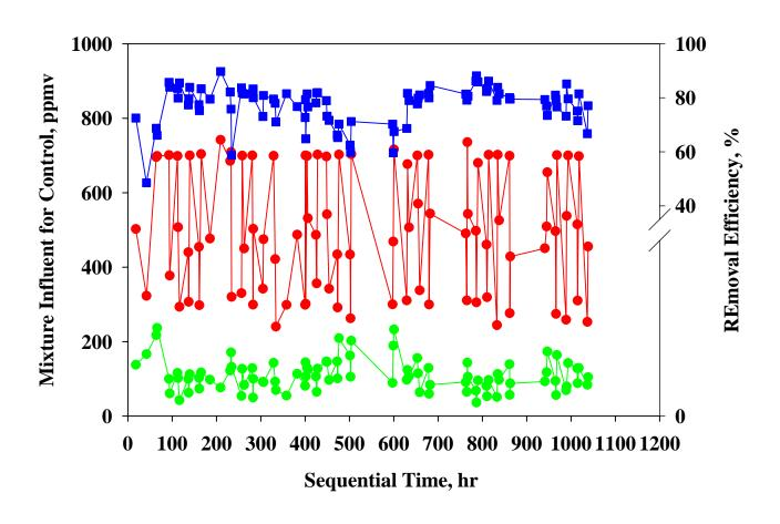
Effective Control of Gaseous VOC Mixture in a TBAB Coupled with Cyclic Adsorption/Desorption Beds
