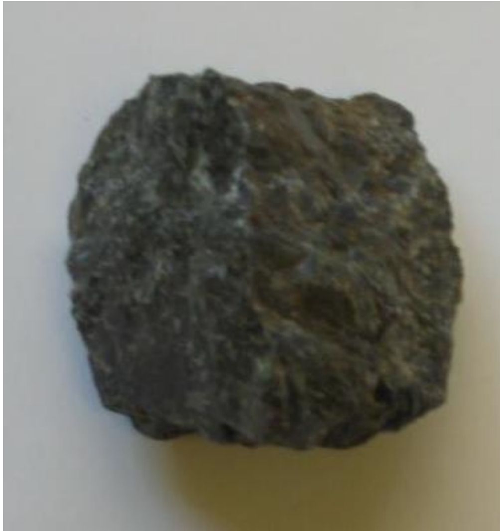
Plagioclase Feldspar - (\text{Ca,Na}),(\text{Al,Si})\text{AlSi}_2\text{O}_8
