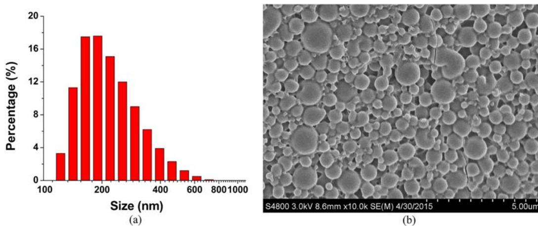
**FIGURE 2.** A, B: Size and morphology of sirolimus-loaded nanoparticles. A: The particle size distribution of the sirolimus-loading nanoparticles measured by a dynamic light scattering instrument (DLS), B: the SEM image showing the surface morphology of sirolimus-loading nanoparticles.
