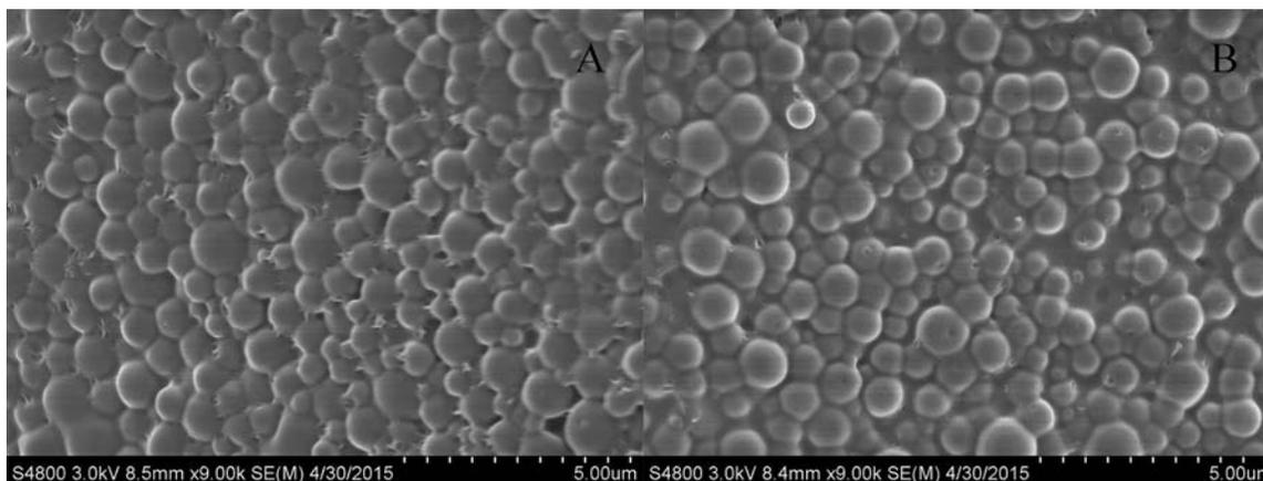
FIGURE 6. A, B: The wash off study of the sirolimus NPs coating: (A) washed for 10 min, and (B) washed for 30 min.
