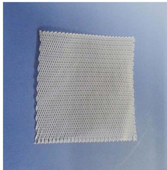
**FIGURE 1.** The 3D printed single layer scaffolds (SLS) with a similar structure of the stents.
