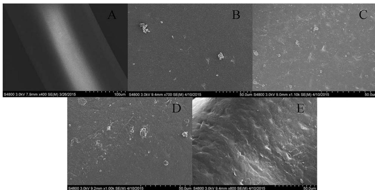
**FIGURE 4.** Surfaces of scaffolds with different plasma treatment. A was the bare stent used as a control; B was the scaffold treated by gaseous polymerization in NVP; C was the scaffold treated by gaseous polymerization in EVA; D was the scaffold treated by liquid polymerization in NVP; E was the scaffold treated by liquid polymerization in EVA.
