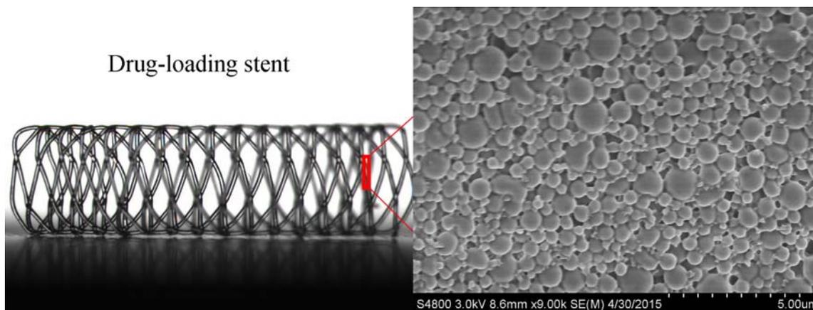
FIGURE 5. The novel biodegradable drug-loaded eluting stent. The SEM picture showing the surface morphology was on the right.
