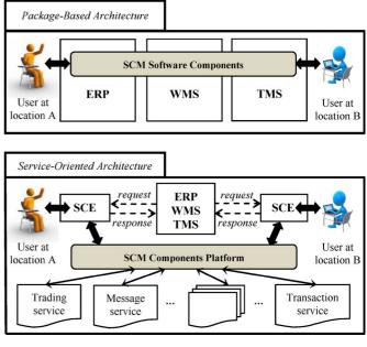
Fig. 4. BXD's SCM software architecture alternatives.
