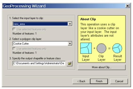
Select the shapefile to be cropped in the top window (ESRI uses the verb "clip" rather than "crop") and the shapefile to crop (clip) to in the middle window. Make sure you specify the name and location of the output (cropped) shapefile in the bottom window. When you press "Finish", a new shapefile cropped to the clipping file will be created and added to the project. Note: the original shapefile will be left unaltered.
