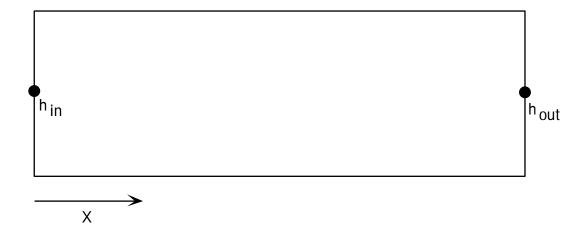
4. (30) Pictured below is the "island problem". Given the values of T, R, and L shown below, determine an analytical expression for head using the Poisson equation  $\left(\frac{d^2h}{dx^2} = -\frac{R}{T}\right)$  and calculate the head at the center of the island.
