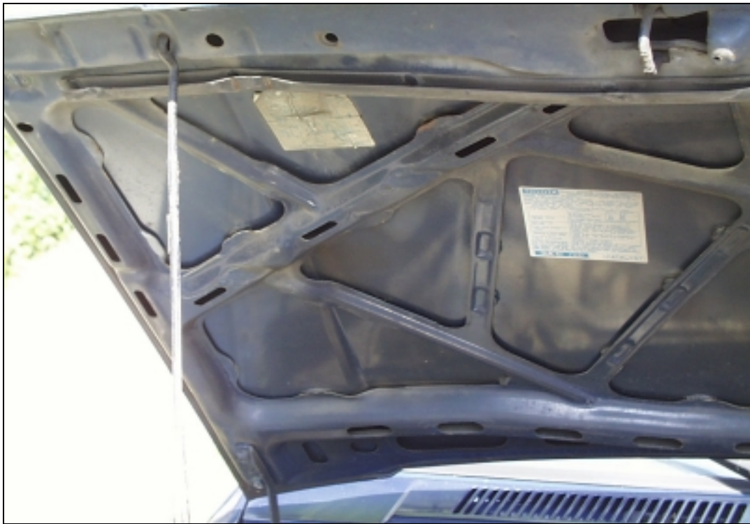
Figure 3. Supporting struts have a higher thermal inertia than the adjacent unsupported sheet metal.
