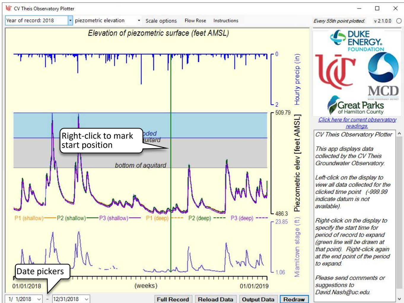
Figure 9 Vertical green line appears at the point the chart is right-clicked at the start date of selected interval. Right clicking at the date corresponding to the end of the selected time period will immediately display the selected interval (Figure 10).
