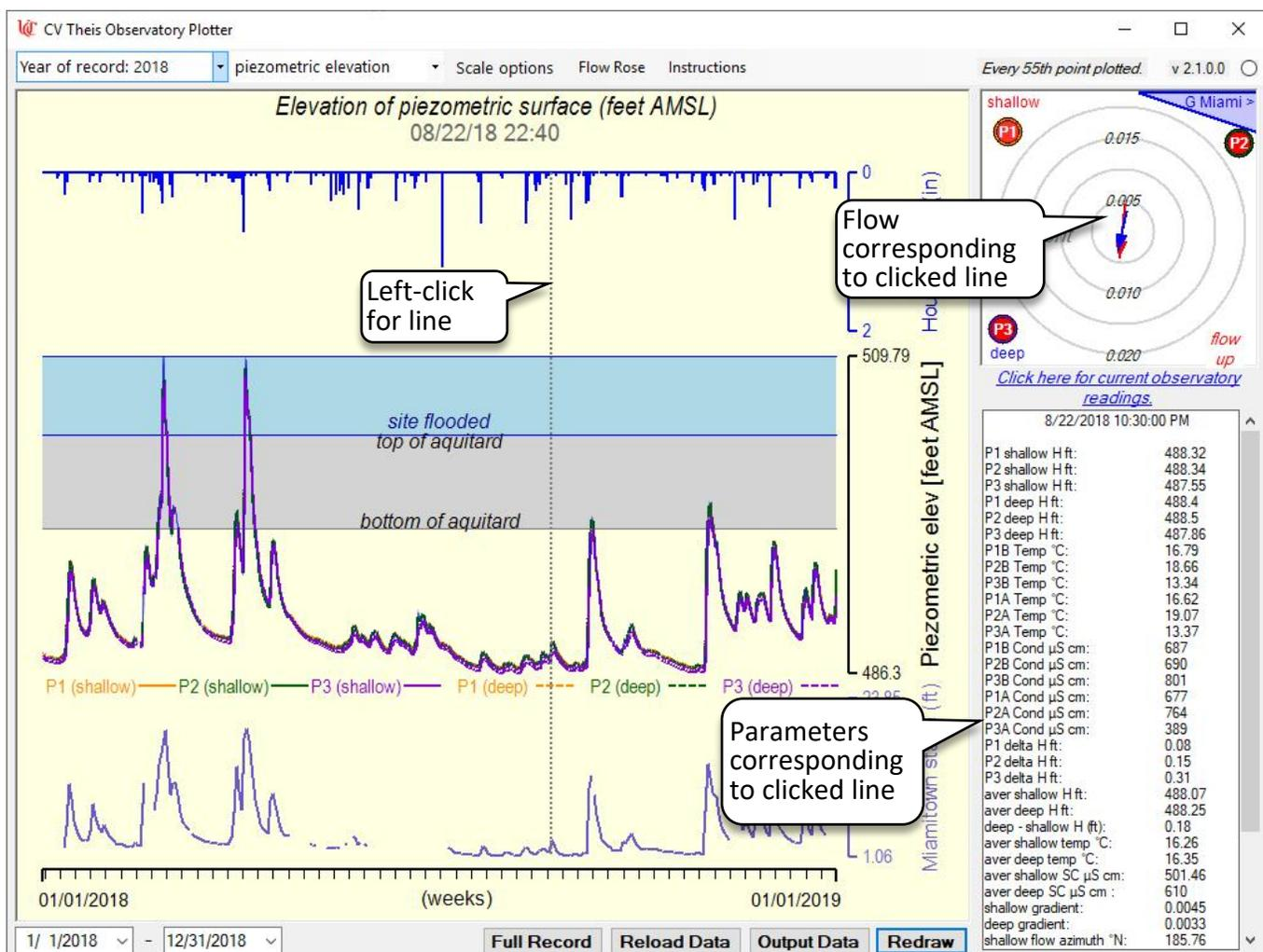
Figure 8 Left-clicking the chart area draws a vertical line at that point and displays the flow dynamics and data corresponding to the clicked point.
