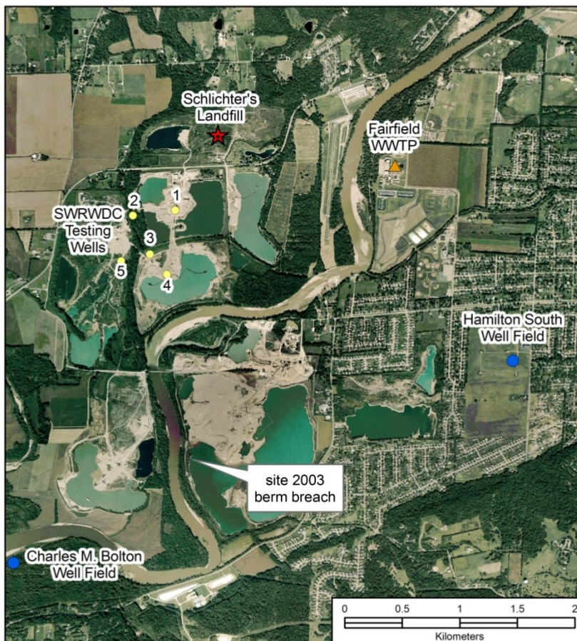
Figure 12. Quarries and abandoned landfills at Hamilton, Ohio. Elevated nitrate and ammonia levels, sometimes exceeding MCL have been detected at SWRWDC observations wells. The contaminants are presumed to have originated from the now-abandoned Schlichter Landfill.
