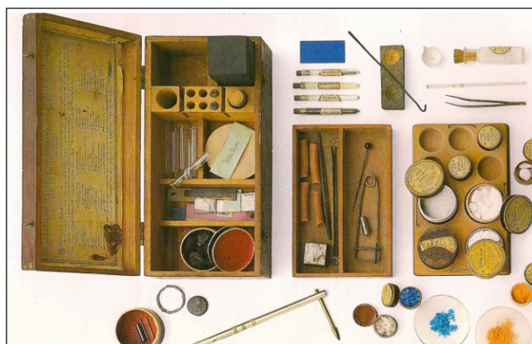
Figure 11. Taylor’s Students’ Guinea Set of Blowpipe Apparatus and Pure Chemical Reagents.
