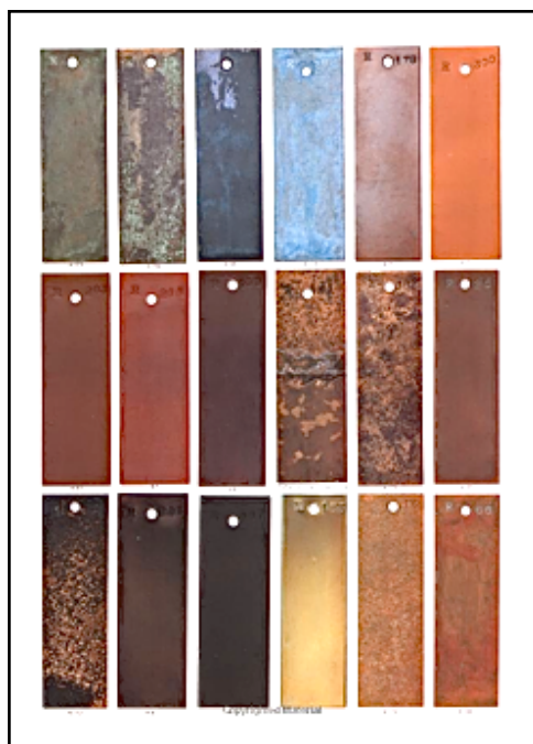
Figure 4. Examples of bronzing effects on an alloy of 90% copper metal and 10% zinc metal (19)
