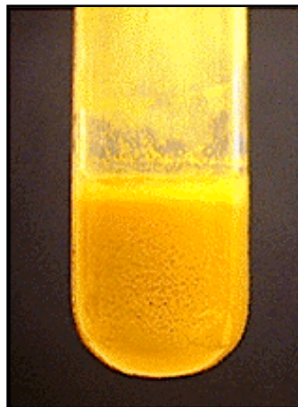
Figure 3. The appearance of tin disulfide when precipitated in the standard qual scheme.
