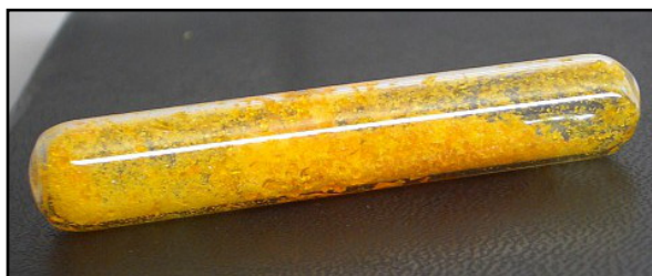
Figure 1. A tube of crystalline hydrogen tetrachloroaurate tetrahydrate. Was this the philosopher's stone?
