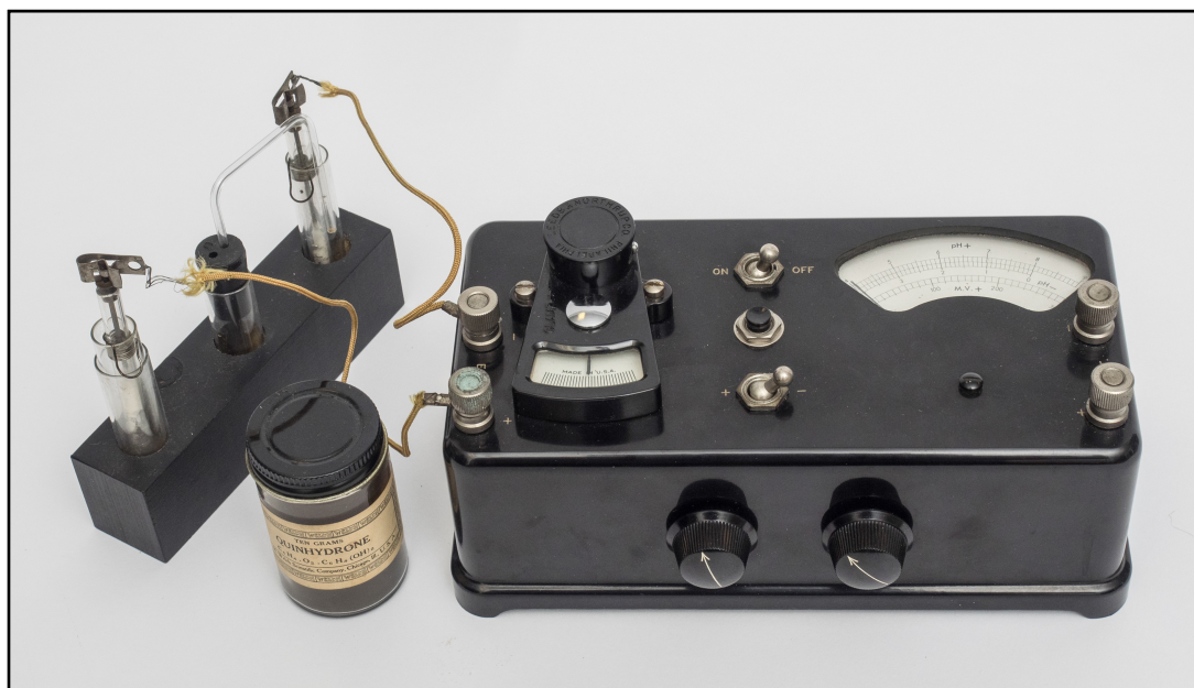
Figure 6. Our recently acquired Youden null-point pH meter. The Moir electrode system, minus one of the salt bridges, is to the left and a circa 1940 bottle of quinhydrone is displayed between it and the meter.
