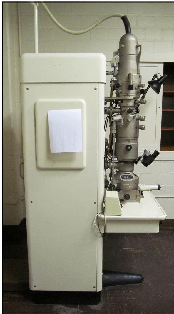
Figure 2. Side view of the Siemens IA Elmiskop in its original location at UC Environmental Health and Safety.
