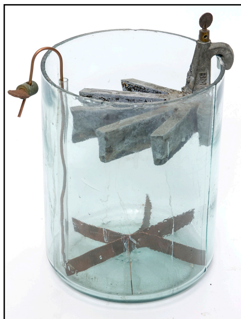
Figure 8. An actual surviving example of the crowfoot form of the Daniell gravity cell shown in figure 7 (Jensen-Thomas Apparatus Collection).
