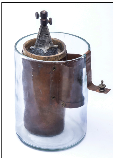
Figure 3. An actual surviving example of the Daniell cell shown in figure 2 (Jensen-Thomas Apparatus Collection).
