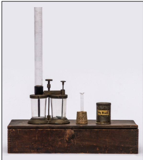
Figure 2. The Twitchell acidometer resting on top of its storage box. From left to right: the acidometer, the calibrated test tube for measuring out vinegar samples, a small tin of potassium bicarbonate for charging the reaction spoon (Jensen-Thomas Apparatus Collection).
