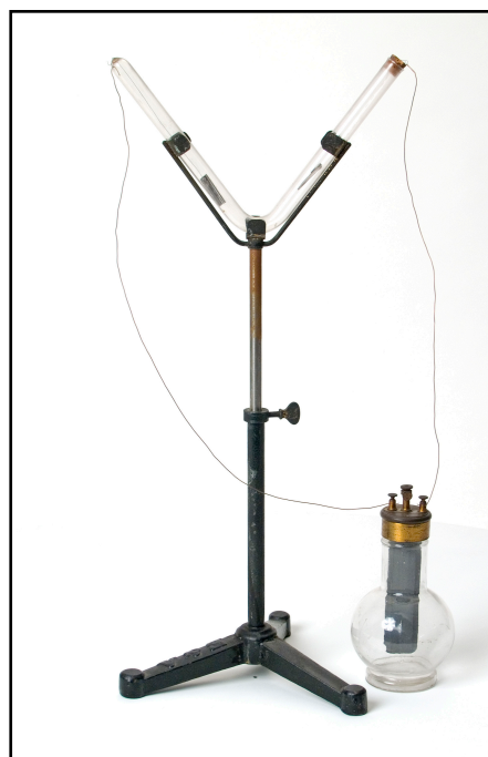
Figure 5. A later version of the Hofmann V-cell for electrolysis. It is being powered by a Grenet dichromate cell (Jensen-Thomas Apparatus Collection).
