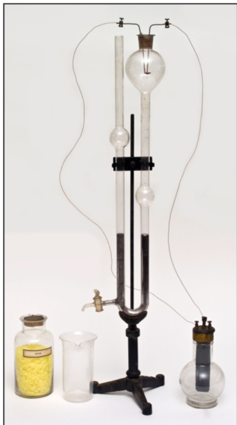
Figure 12. A later example of a Hofmann eudiometer used for demonstrating volume changes in solid-gas reactions. The glass stopper at the top of the bulb is missing (Jensen-Thomas Apparatus Collection).
