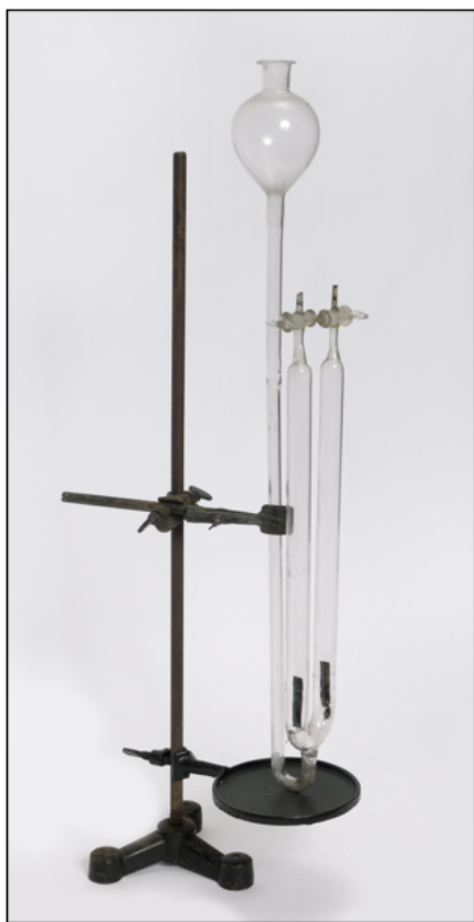
Figure 7. A later version of the Hofmann U-cell for electrolysis based on his final design of 1869 (Jensen-Thomas Apparatus Collection).
