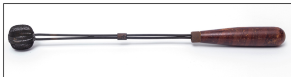
Figure 3. A later version of the Hofmann sodium spoon (Jensen-Thomas Apparatus Collection).
