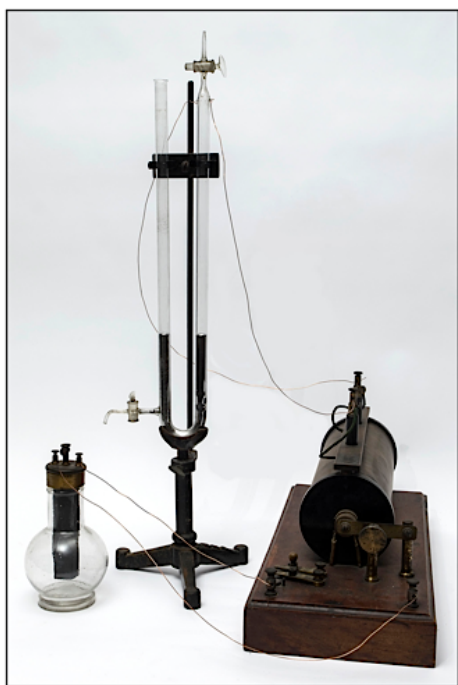
Figure 10. A later version of a Hofmann eudiometer used for demonstrating the volume changes in gas-gas reactions (Jensen-Thomas Apparatus Collection).
