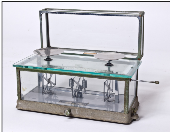
Figure 11. An example of a Springer-Roeder torsion balance from the Oesper Collections. The three pivot frames with their X-supports and the two columns of weights on either side of the lower beam's pivot point are clearly visible through the all-glass case.
