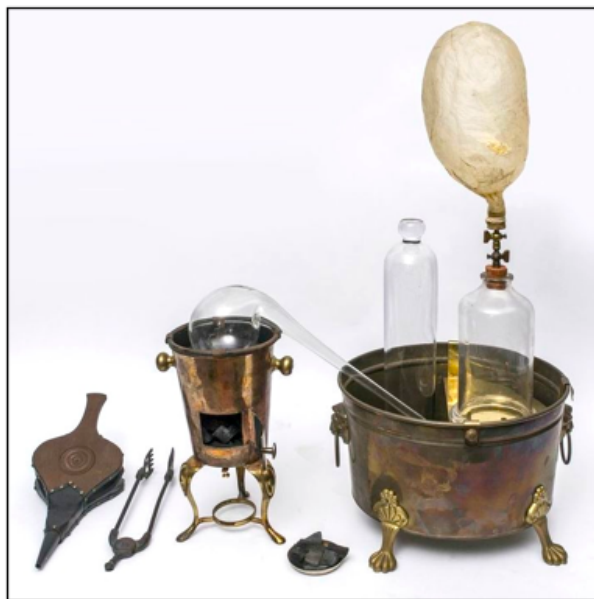
Figure 10. Reproduction of an 18th-century retort, pneumatic trough, and charcoal furnace similar to those used by Lavoisier (Jensen-Thomas Apparatus Collection).
