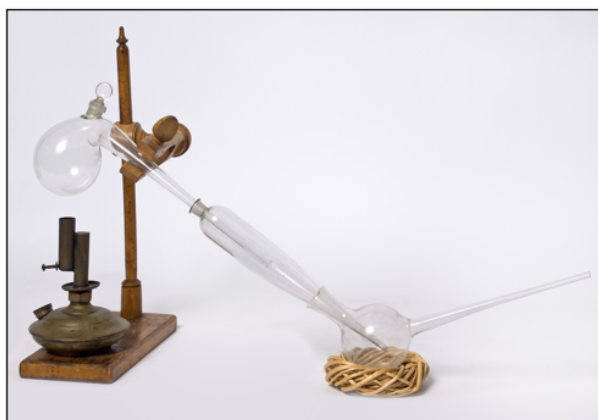
Figure 12. Medium retort with adapter and quilled receiver (Jensen-Thomas Apparatus Collection).
