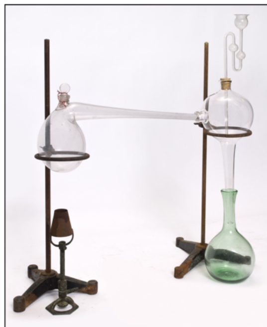
Figure 13. Large retort with an alternative orientation for a quilled receiver fitted with a safety tube (Jensen-Thomas Apparatus Collection).
