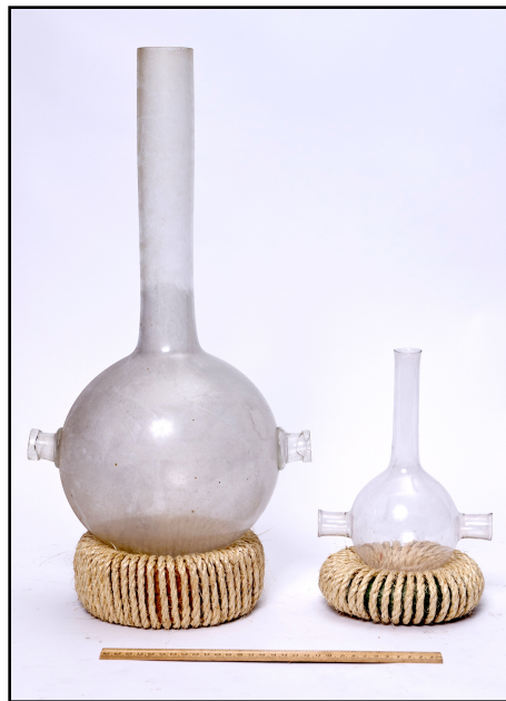
Figure 14. Examples of tubulated retort receivers of varying sizes and ages (Jensen-Thomas Apparatus Collection).
