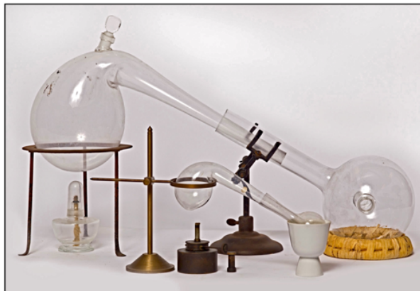
Figure 9. Range of glass retort sizes illustrated using a 1.5 L, c. 1860, lime-glass, tubulated retort and tubulated receiver and a 25 mL, c. 1900, soft glass, plain retort with a plain receiver (Jensen-Thomas Apparatus Collection).
