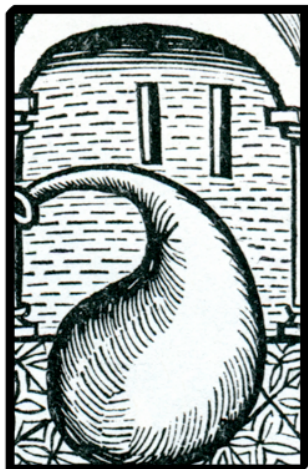
Figure 4. An early woodcut of a retort from the 1512 edition of Brunschwigk's famous book on distillation.
