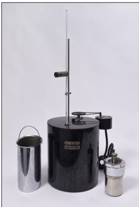
Figure 6. An example of a Parr oxygen bomb calorimeter, c. 1940 (Jensen-Thomas Apparatus Collection).
