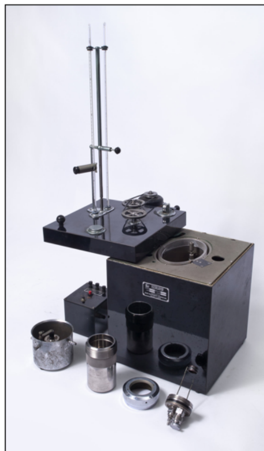
Figure 7. An example of a Parr adiabatic oxygen bomb calorimeter, c. 1956 (Jensen-Thomas Apparatus Collection).
