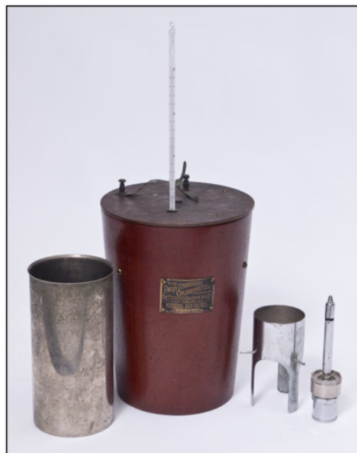
Figure 4. An example of a later variant of the Parr peroxide calorimeter, c. 1912 (Jensen-Thomas Apparatus Collection). The water chamber is to the left and the combustion bomb and pivot support are to the right. The pulley attachment for the top of the combustion bomb and the detachable stirring wings are missing.
