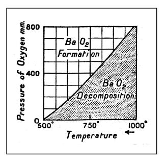
Figure 1. A plot of pressure versus temperature showing the regions corresponding to the favorable production of barium oxide versus barium peroxide (7).
