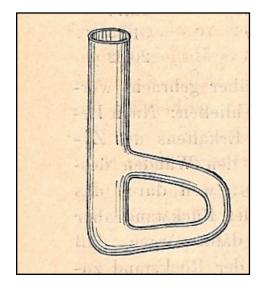
Figure 2. Thiele's original melting point tube, circa 1907 (7).
