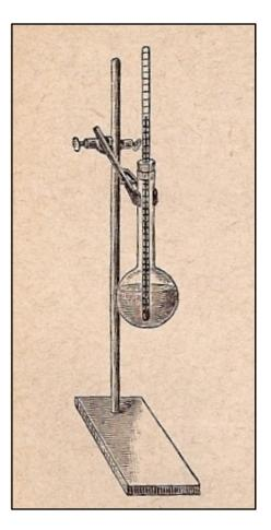
Figure 1. Simple melting-point apparatus as depicted by Gattermann in 1894 (6).
