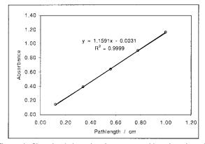
Figure 1. Plot of solution absorbance vs pathlength, using glass spacers. The least-squares fit equation and  $R^2$  value are included. The absorbance was measured with a Shimadzu UV 260 dual-beam spectrophotometer at 470 nm for 0.00352 M  $I_2$  in 0.00941 M KI.
