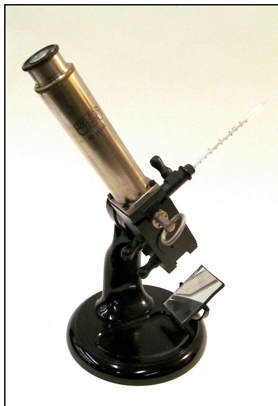
Figure 2. A circa 1920 Zeiss Butter Refractometer.
