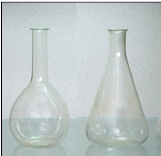
Figure 4. 19th-century examples from the Oesper Collections of a round Florence flask (left) and a conical Erlenmeyer flask (right), both made of lime or Bohemian glass.
