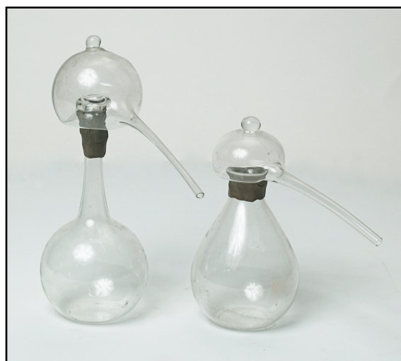
Figure 3. Two replicas of small, flat-bottom alembics with clay luting (Jensen-Thomas Apparatus Collection).
