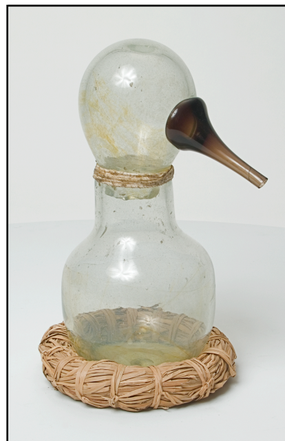
Figure 2. A handblown replica of an early alembic with a broken beak and a woven straw support ring (Jensen-Thomas Apparatus Collection). Note the absence of a collection gutter.
