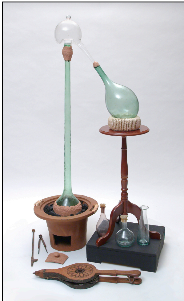
Figure 4. A reproduction of a circa 17th-century alembic with an “ostrich”-necked cucubert, clay luting, various receiving flasks, charcoal furnace, bellows, tongs, and poker (Jensen-Thomas Apparatus Collection).
