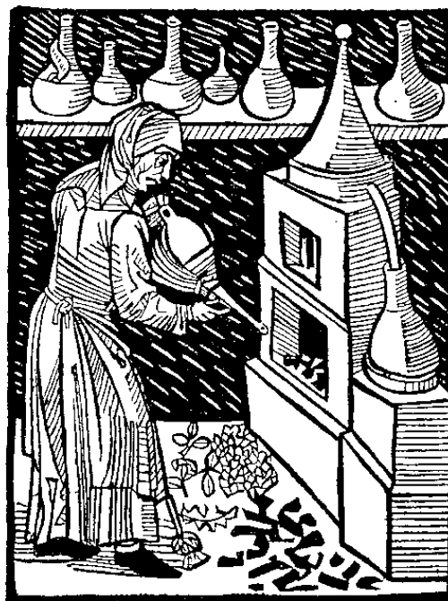
Figure 5. A Rosenhut as pictured on the title page of Puff von Schrick’s 1474 booklet on the distillation of flavored brandies. The copper cone on top of the furnace is the Rosenhut or condensing head. The cucubert is hidden within the furnace itself.
