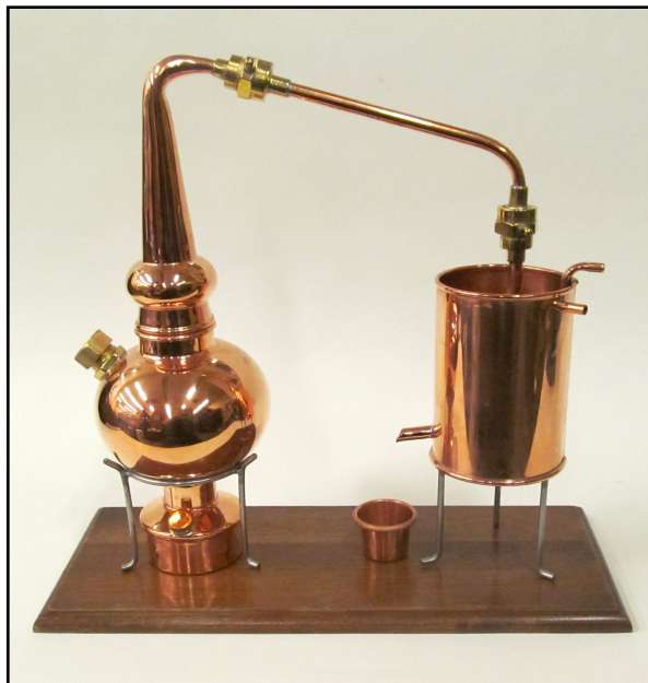
Figure 8. A working desktop model of a copper alembic with a water-cooled coil condenser like those used for industrial-scale distillation (Jensen-Thomas Apparatus Collection). Once again the condensing coil is hidden from view in the cylindrical container to the right through which the cooling water circulates.
