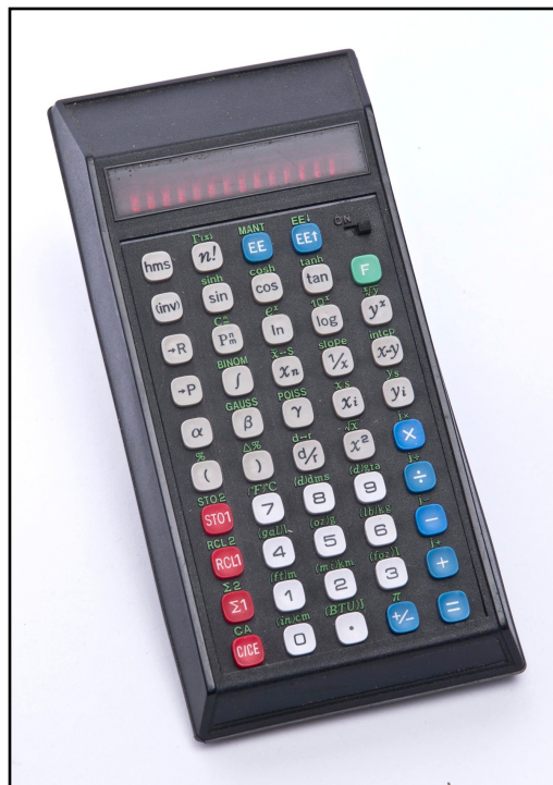
Figure 5. A more sophisticated, circa late-1970s, portable electronic calculator with a LED display.
