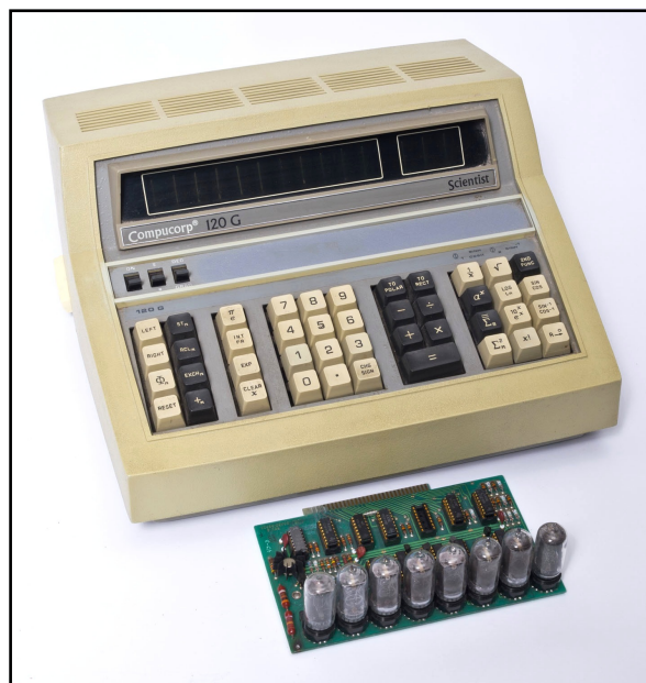
Figure 3. A circa 1971 electronic “Compucorp” calculator using a Nixie tube display. An example array of Nixie tubes is shown in the foreground.
