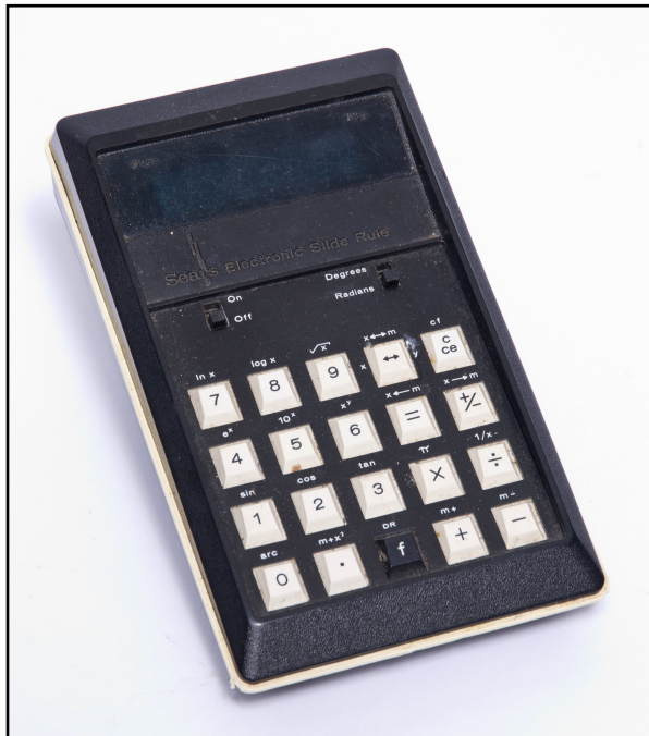
Figure 4. A circa mid-1970s portable electronic calculator with a LED display marketed by Sears under the logo “Electronic Slide Rule.”
