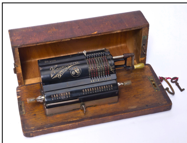
Figure 1. A circa 1920 German-made “Hannovera” hand-cranked mechanical calculator and its wooden storage case.
