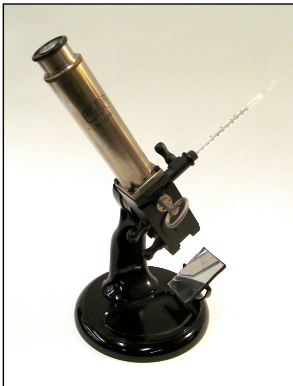
Figure 3. The circa 1920 Zeiss butter refractometer recently acquired by the Oesper Collections. It is shown with the cell compartment closed and no rubber tubing attached to the water nipples. The micrometer screw, which is to the left of the optical tube, is not visible in this photo.
