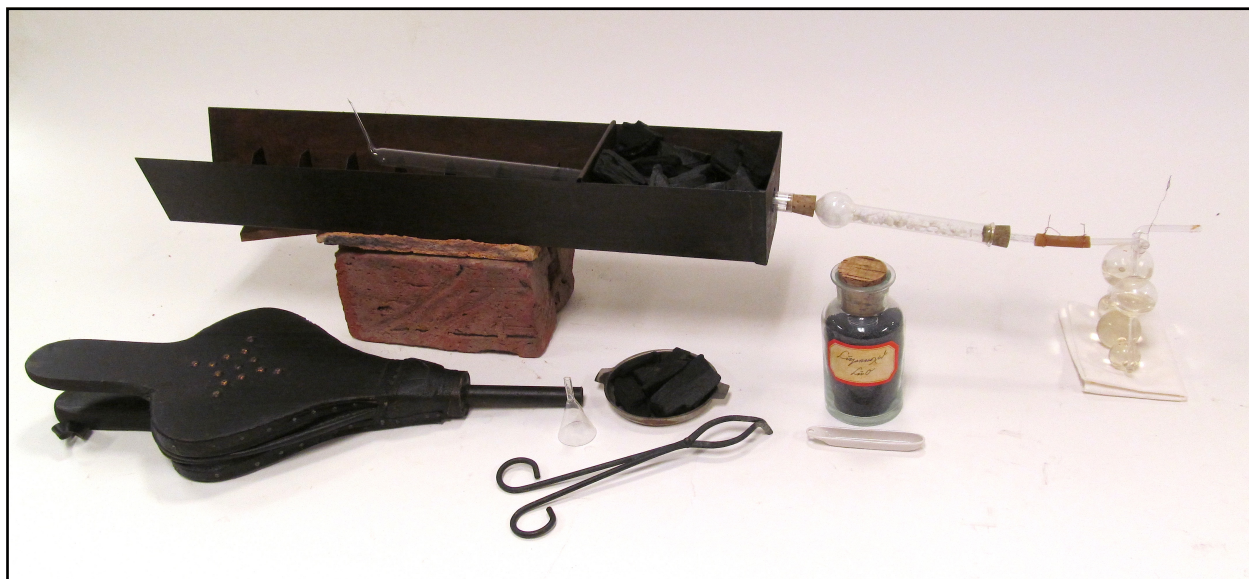
Figure 7. A reproduction of Liebig's original apparatus for combustion analysis based on Dr. Usselman's gift. Background (left to right) : charcoal furnace and combustion tube, calcium dichloride tube, Kali bulb. Foreground (left to right) : bellows and small funnel for filling the Kali bulb, extra charcoal and tongs, bottle of copper oxide and a porcelain combustion boat (Jensen-Thomas Apparatus Collection). Compare with figure 3.
