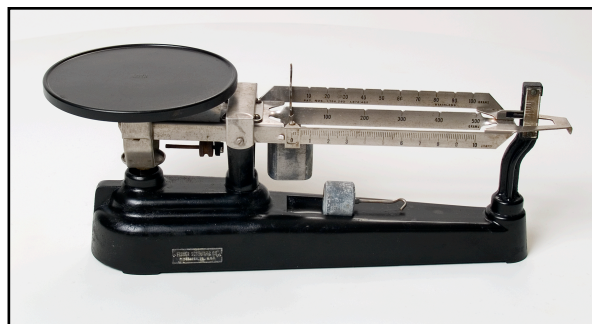
Figures 5 and 6. Examples of circa 1940 triple-beam laboratory balances based on the steelyard principle. Top : A triple-beam balance with a traditional suspended pan sold by Welsh Scientific. Bottom : A triple-beam platform balance sold by Fisher Scientific with the pan mounted on top of, rather than suspended below, the beam (Jensen-Thomas Apparatus Collection).
