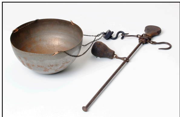
Figure 4. A medium-size late 19th-century commercial steelyard with a 18.5” beam (Jensen-Thomas Apparatus Collection).
