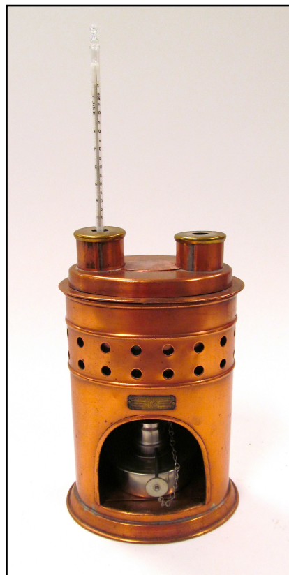
Figure 3. The restored 1913 Foster flashpoint apparatus.
