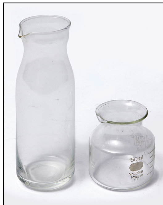
Figure 3. Typical “fleakers,” both old (left) and new (right) from the Jensen-Thomas Apparatus Collection.
