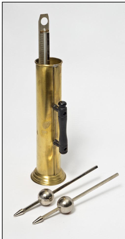
Figure 2. A brass hydrometer jar with handle and thermometer and two metal hydrometers probably designed to monitor the fermentation of beer (Jensen-Thomas Apparatus Collection). The handle would facilitate scooping samples from the open beer vats.
