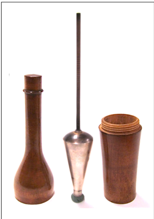
Figure 4. Twitchell's (1.25" x 7.75") metal hydrometer for determining the alcohol content of wine and spirits.
