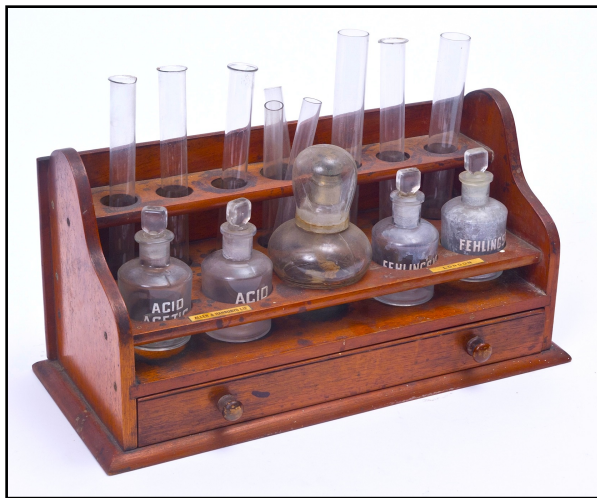
Figure 5. An early 20th-century physician's office kit for testing urine for sugar using Fehling's solution (Jensen-Thomas Apparatus Collection). The two bottles on the left contained the dilute acids required to hydrolyze any sucrose present to glucose and fructose. The two bottles on the right, labelled Fehling's solution, contained the copper tartrate complex and the sodium hydroxide solution, respectively, that had to be freshly mixed before performing the actual test.
