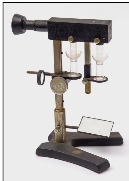
Figure 6. A circa 1928 Bock-Benedict colorimeter (Jensen-Thomas Apparatus Collection).
