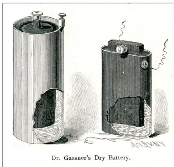
Figure 7. A circa 1890 etching of two of Gassner's early dry cells. The gap between the outer Zn case and the central MnO 2 /C cathode containing the electrolyte paste is clearly visible in each case.
