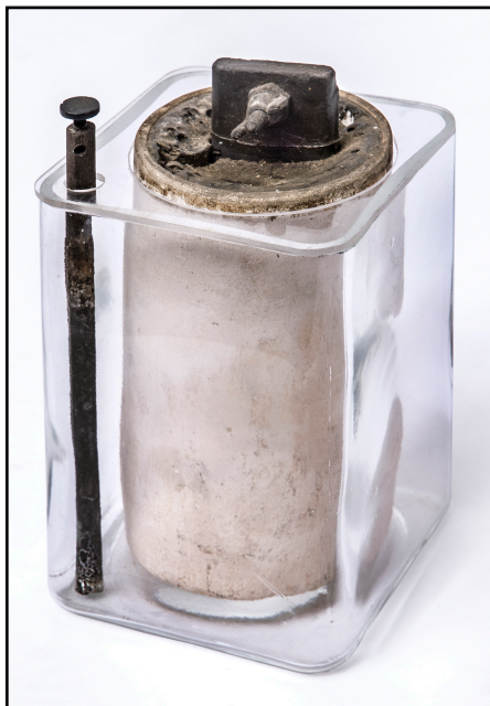
Figure 3. An example of an early Leclanché cell similar to that in figure 2 (Jensen-Thomas Apparatus Collection).
