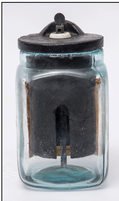
Figure 6. The cell in figure 5 shown from the back so as to more clearly display the cylindrical MnO 2 /C cathode and the central Zn rod anode.
