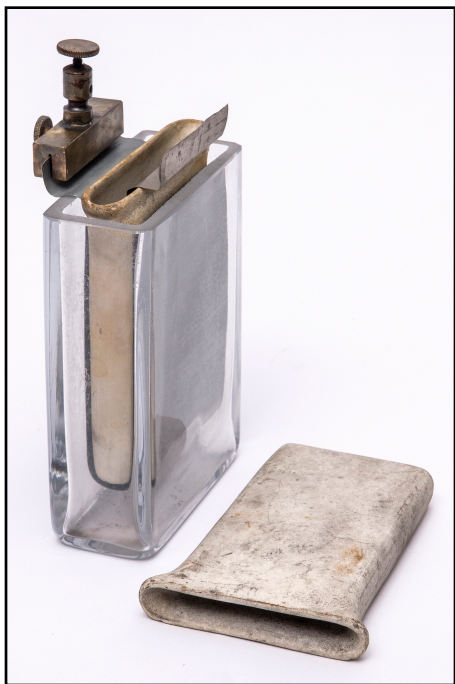
Figure 3. An actual surviving example of the Grove cell shown in figure 2 (Jensen-Thomas Apparatus Collection) and a spare ceramic spacer.
