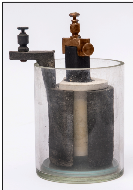
Figure 8. An actual surviving example of the Bunsen carbon cell shown in figure 7 (Jensen-Thomas Apparatus Collection).
