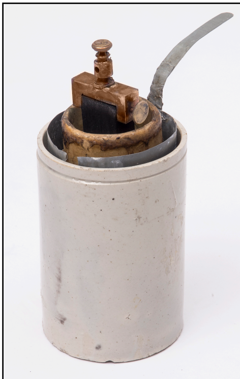
Figure 6. A example of a Bunsen carbon cell like that that shown in figure 5 (Jensen-Thomas Apparatus Collection).
