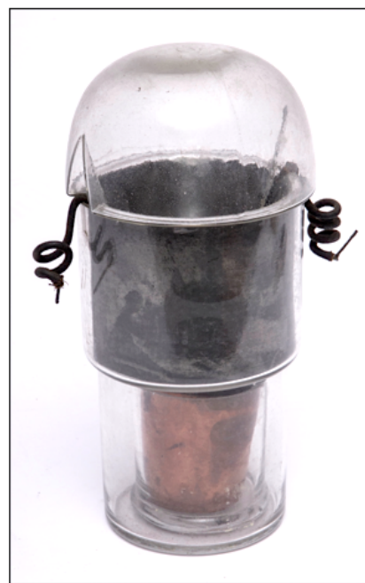
Figure 5. An actual surviving example of the globe or Meidinger form of the Daniell cell shown in figure 4 (Jensen-Thomas Apparatus Collection).
