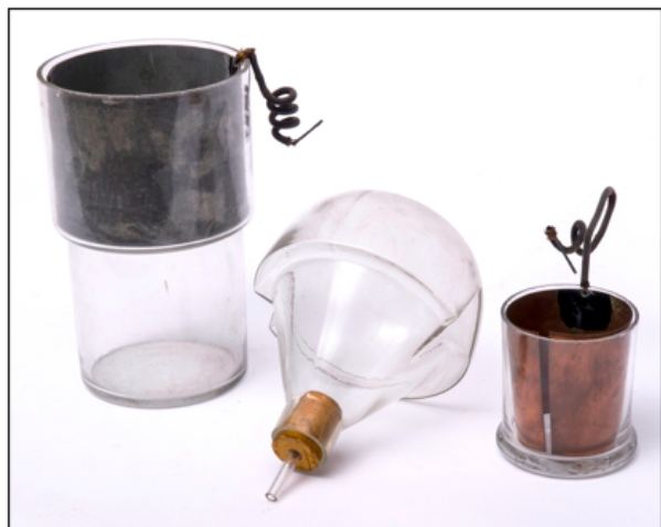
Figure 6. A disassembled Meidinger cell. From left to right: The outer cylinder and Zn anode, the globe or \text{Cu}(\text{SO}_4)(\text{s}) reservoir, the inner cup and Cu cathode.
