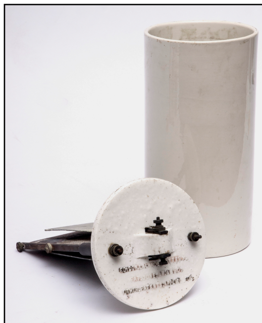
Figure 2. An Edison-Lalande cell (Jensen-Thomas Apparatus Collection). The embossed printing on the ceramic lid reads "Edison Lalande Battery, Patented June 17, 1890. Other Patents Applied For." The central plate is the \text{Cu}/\text{CuO} cathode and those on either side are the \text{Zn} anodes.
