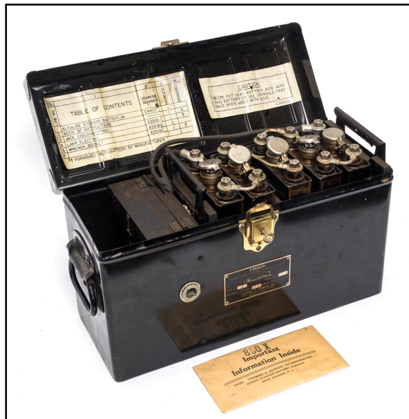
Figure 4. An almost pristine three-cell battery pack of nickel-iron storage cells ready for installation in an electric car (Jensen-Thomas Apparatus Collection).
