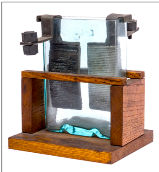
Figure 2. A Planté lead cell (Jensen-Thomas Apparatus Collection). This setup was for demonstration purposes only and the commercial version in your car battery has a far more complex electrode configuration. The number of such cells in older car batteries could be determined by simply counting the number of openings for replenishing the \text{H}_2(\text{SO}_4) electrolyte in each cell compartment.
