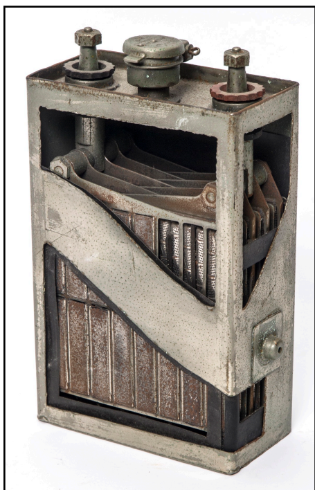
Figure 3. A cutaway of the final commercial version of Edison's nickel-iron alkaline storage battery (Jensen-Thomas Apparatus Collection). The nine interleaved plates are not separate cells but are rather a way of increasing electrode surface area.
