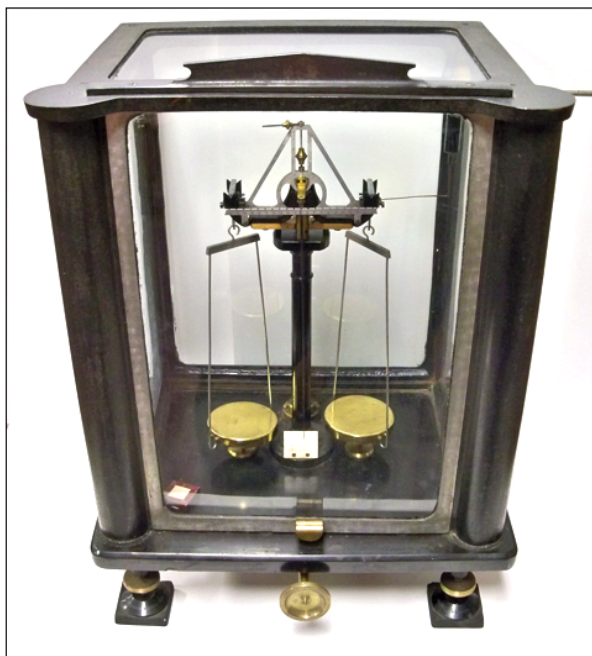
Figure 4. A recently acquired Bunge style short-beam analytical balance with a cast-iron case, black-glass base, and triangulated aluminum beam, circa 1885 (Jensen-Thomas Apparatus Collection).
