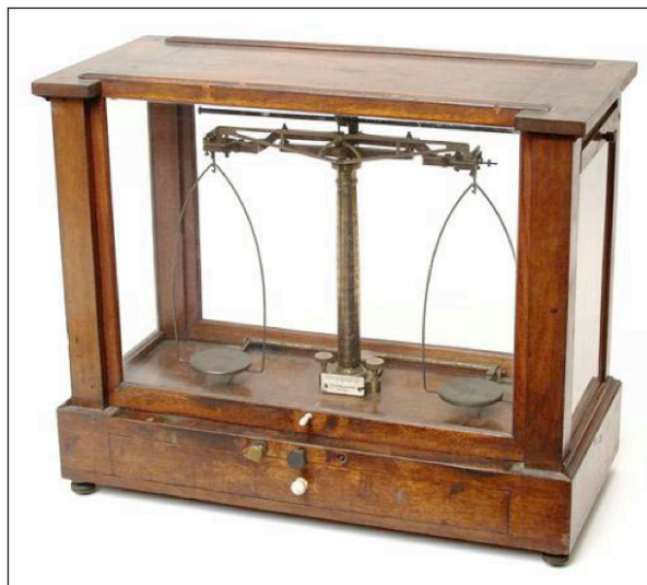
Figure 2. A Becker long-beam balance, c. 1860 (Jensen-Thomas Apparatus Collection).
