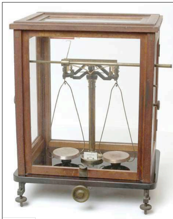
Figure 3. A Bunge style short-beam balance made by Sartorius, c. 1875 (Jensen-Thomas Apparatus Collection).
