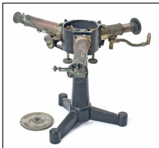
Figure 15. Brass spectroscope in the Oesper Apparatus Collections on which the tile in figure 13 is based. As depicted on the tile, parts of the spectroscope have been cut away to reveal the glass prism inside.
