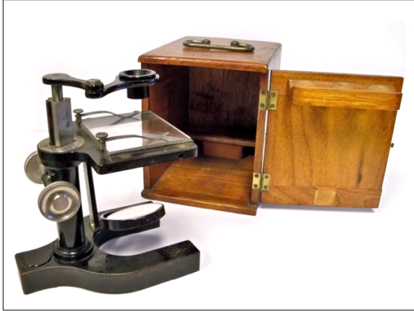
Figure 3. A single-lens Bausch and Lomb student dissecting microscope, c.1930 (Jensen-Thomas Apparatus Collection).
