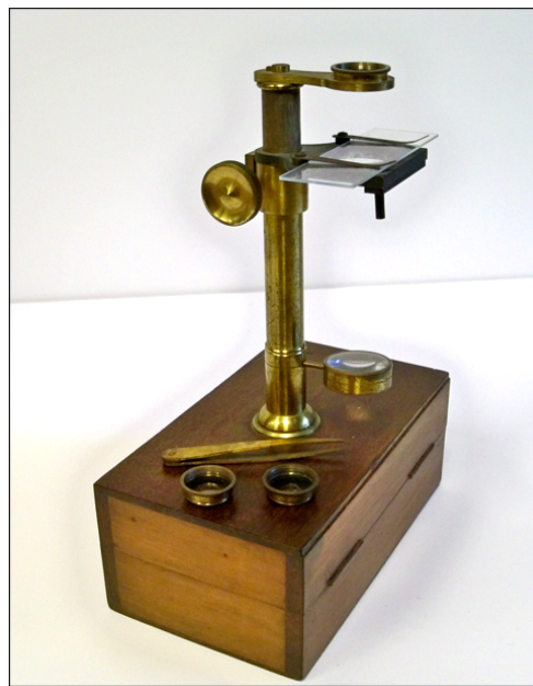
Figure 1. The single-lens microscope donated to the Jensen-Thomas Apparatus Collection by Dr. O. B. Ramsay.
