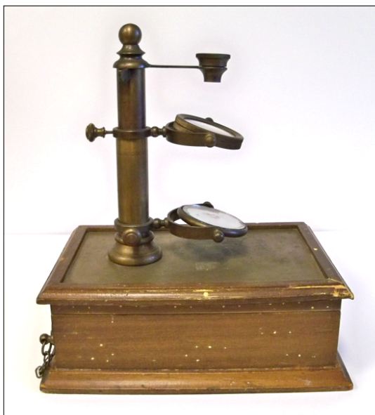
Figure 2. The reproduction of the single-lens microscope used by Charles Darwin during the voyage of the HMS Beagle (Jensen-Thomas Apparatus Collection).
