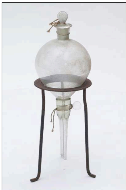
Figure 2. A traditional separatory funnel, c. 1880. (Jensen-Thomas Apparatus Collection).
