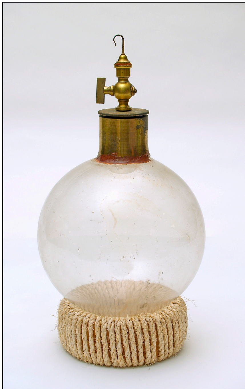
Figure 24. A 19th-century, 8 L, glass balloon with brass stopcock and weighing hook for the determination of gas densities. Compare with figures 3 and 4.
