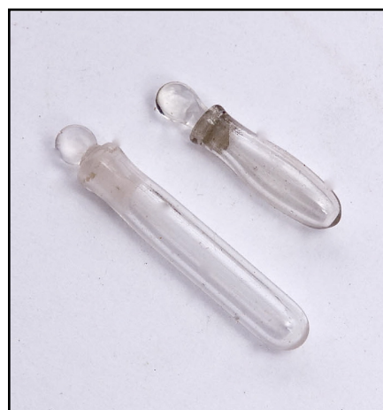
Figure 28. Left: A circa 1900 (11.5" x 18" x 37") Victor Meyer apparatus for the determination of vapor densities. Above: Close-up of (0.19" x 1.25" and 0.13" x 0.88") vials for introducing liquid samples into the Victor Meyer apparatus. Compare with figure 8.
