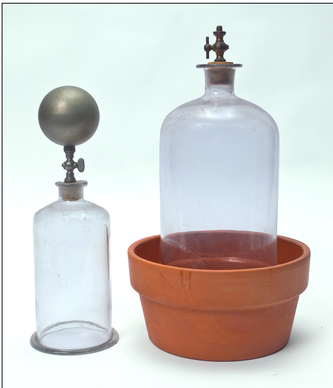
Figure 25. Gas receivers. The (6" x 16.5") example on the left is attached to a small metal balloon, whereas the (12" x 21") example on the right is sitting in an earthenware transfer basin. Compare the figure 3.
