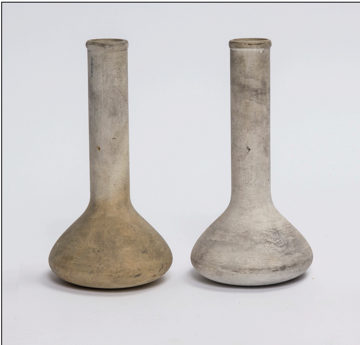
Figure 36. Unglazed (3" x 6") porous ceramic flasks for use as high pressure osmosis cells after the manner of Pfeffer. These are listed twice in the circa 1920 catalog for the laboratory supply house of John J. Griffin and Sons of London – once under the heading of osmosis flasks and once under the heading of filter flasks.
