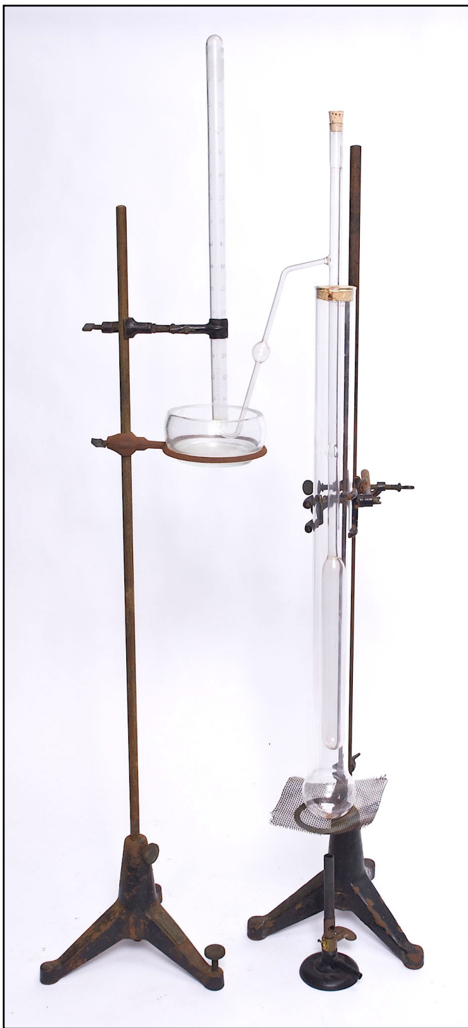
Figure 28. Left: A circa 1900 (11.5" x 18" x 37") Victor Meyer apparatus for the determination of vapor densities. Above: Close-up of (0.19" x 1.25" and 0.13" x 0.88") vials for introducing liquid samples into the Victor Meyer apparatus. Compare with figure 8.
