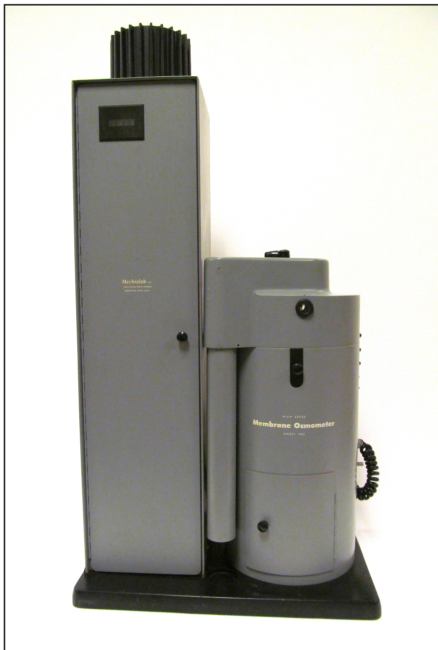
Figure 38. A circa 1970 (12" x 18" x 35") automated membrane osmometer made by Mechrolab Inc. of Mountain View, California. Shown sans power control and printer. Designed to measure average molecular weights between 20,000 and 1,000,000. See also figure 40.
