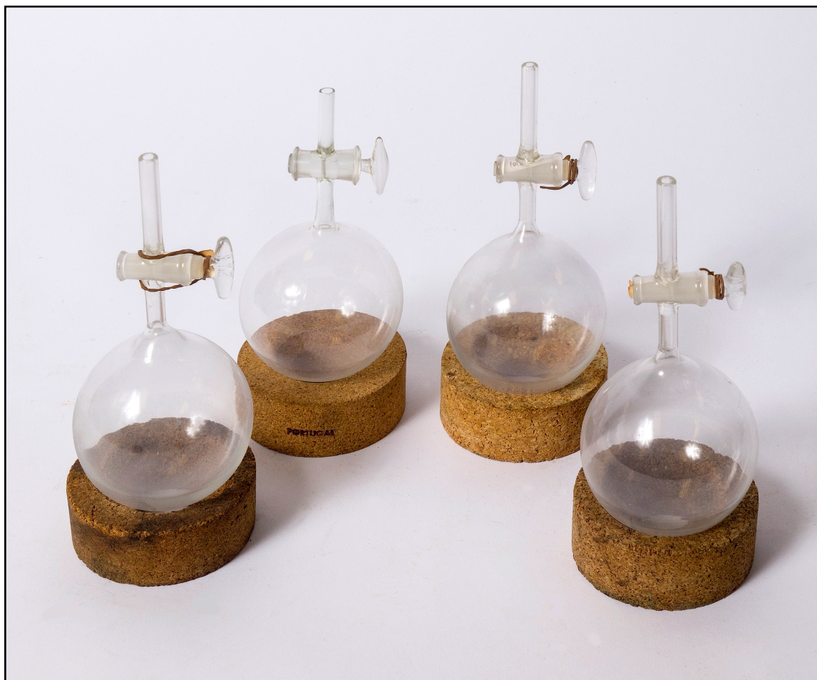
Figure 26. Circa 1960, 150 mL glass bulbs with glass stopcocks for the determination of gas densities, largely as an exercise for the undergraduate physical chemistry laboratory.
