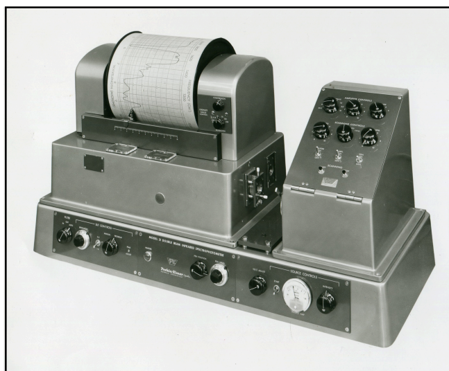
Figure 30. The rather bulky circa 1951 “Model 21 Double-Beam Infrared Spectrophotometer” made by Perkin-Elmer. This was in fact compact compared to the earlier Perkin-Elmer Model 12-C and the Beckman IR-3.
