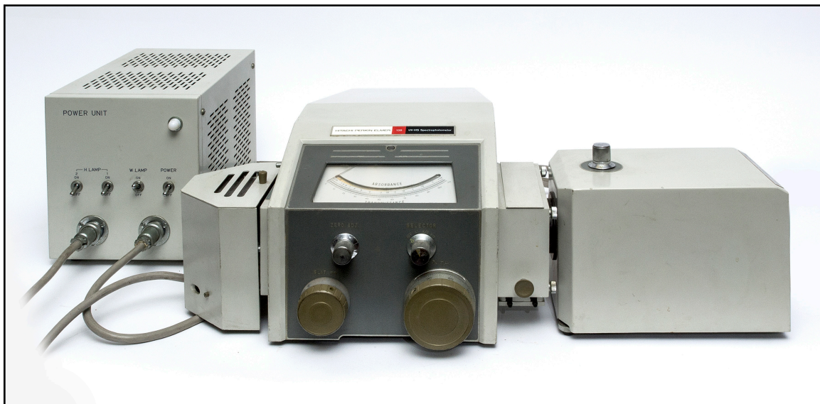
Figure 43. A circa 1963 (34.5" x 21" x 9.25") "Hatischi Model 139 UV-Visible Spectrophotometer" made by Perkin-Elmer of Norwalk CT. Compare with figure 19.
