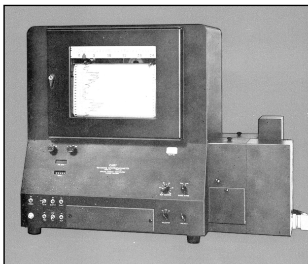
Figure 25. The circa 1947 Cary-11 recording UV-visible spectrophotometer.
