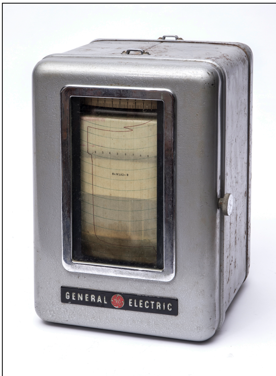
Figure 45. A circa 1950 (13.25" x 9.5" x 8.75") portable electric chart-recorder made by General Electric of Schenectady, NY. Whether it ever occurred to anyone to connect this particular model to a spectrophotometer is unknown. Most photos from the 1950s show the use of massive floor-model recorders instead.
