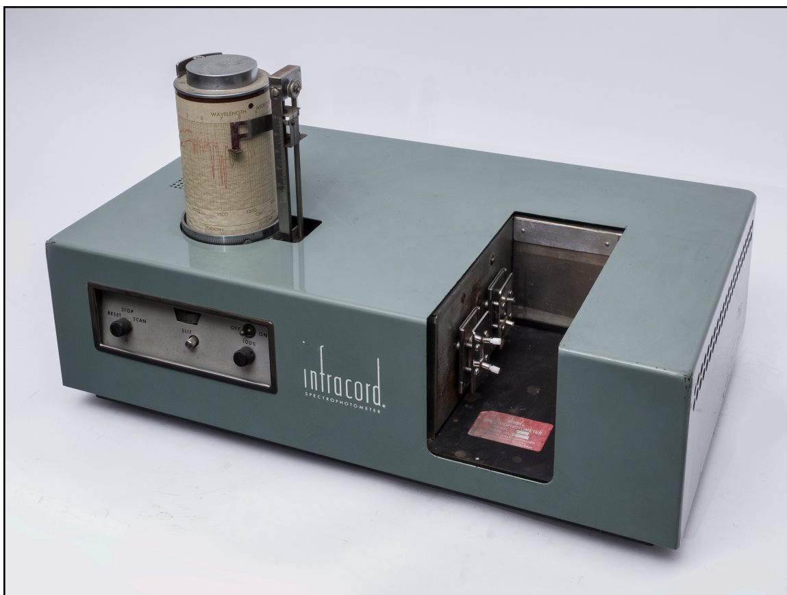
Figure 46. A circa 1958 (27" x 18.75" x 16.75") "Model 137 Infracord" recording IR spectrophotometer made by the Perkin-Elmer Corporation of Norwalk, CT
