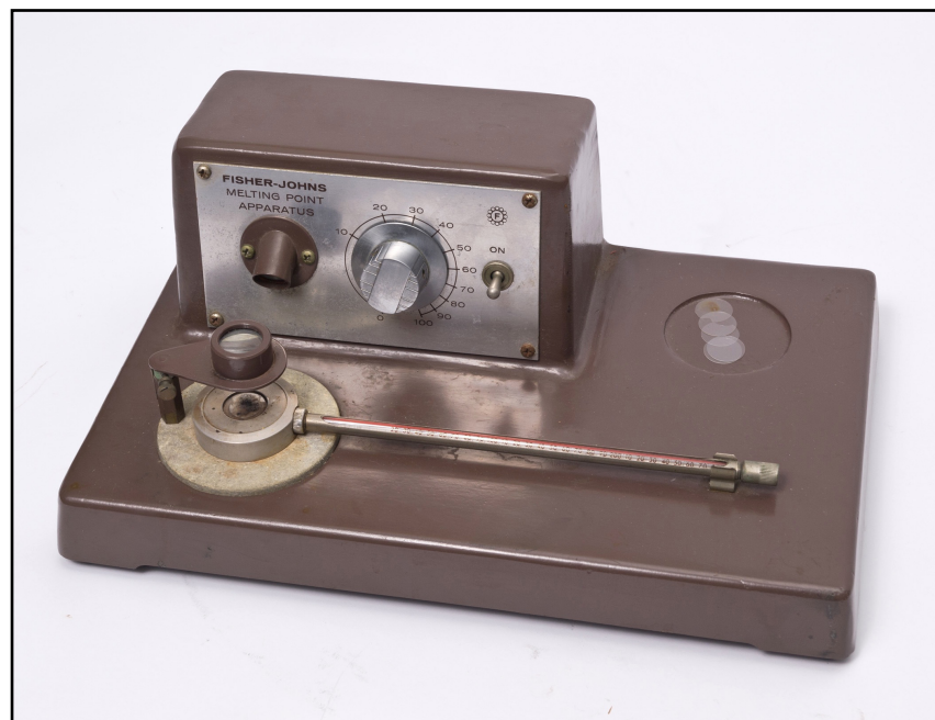
Figure 18. A surviving example of a circa 1960 horizontal (14" x 8.75" x 5.75") electric Fisher-Johns melting-point apparatus similar to that shown in figure 17.
