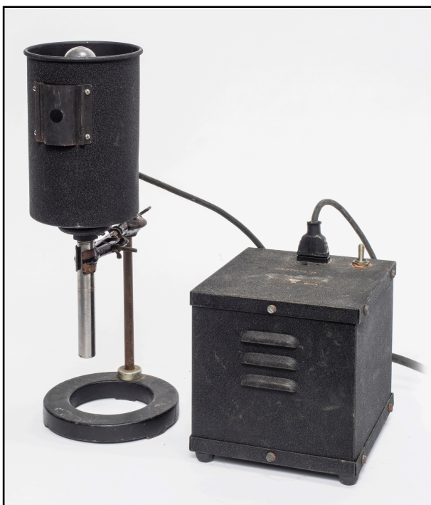
Figure 23 ( left ). A circa 1950 sodium vapor lamp and power source (power source: 6" x 6" x 5.75"; lamp & stand: 14" x 8" x 5"). No manufacturer information is indicated on either the lamp or the power source.
