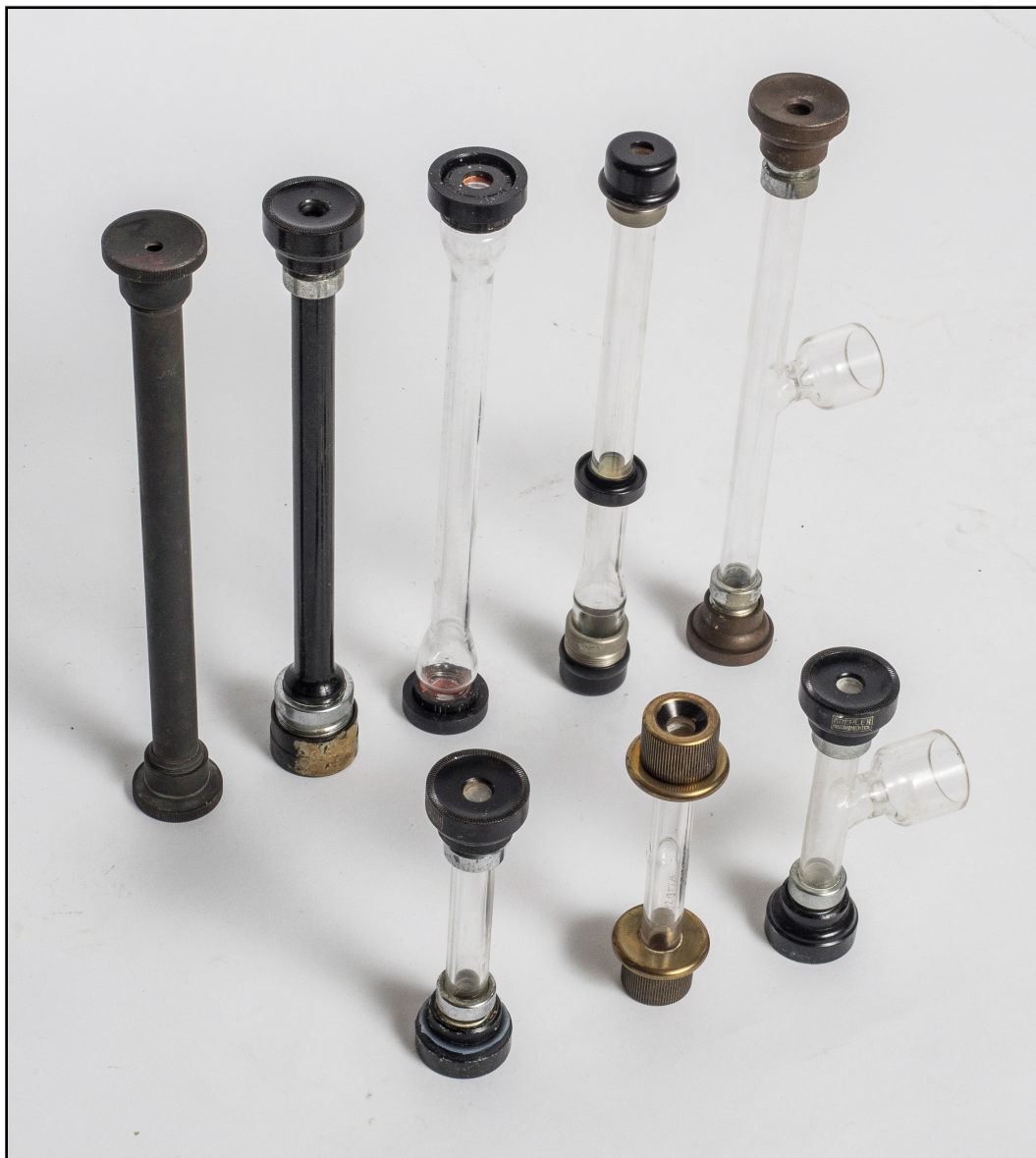
Figure 18. A selection of polarimeter tubes. They range in size from 8.25" x 1" to 4.25" x 1". Some are encased in metal, some have tinted glass, and some have a side opening for adding the sample and/or monitoring the temperature. The caps on the older tubes are metal whereas those on the newer tubes are plastic.
