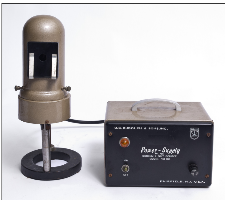
Figure 24 ( right ). A circa 1960 sodium vapor lamp and power source (power source: 15" x 8" x 5.5"; lamp & stand: 15" x 8" x 5"). The power source indicates that it was manufactured by O. C. Rudolph & Sons, Inc. of Fairfield, NJ, as Model No. 90.
