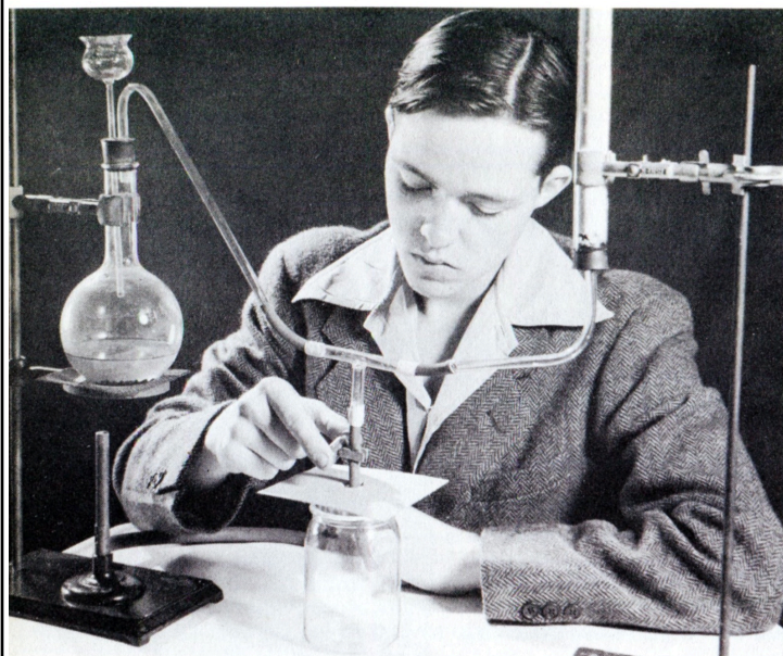
Chlorine is generated in the flask and flows into the center jar when the pinchcock is open. Waste goes into the scrubbing tube.
