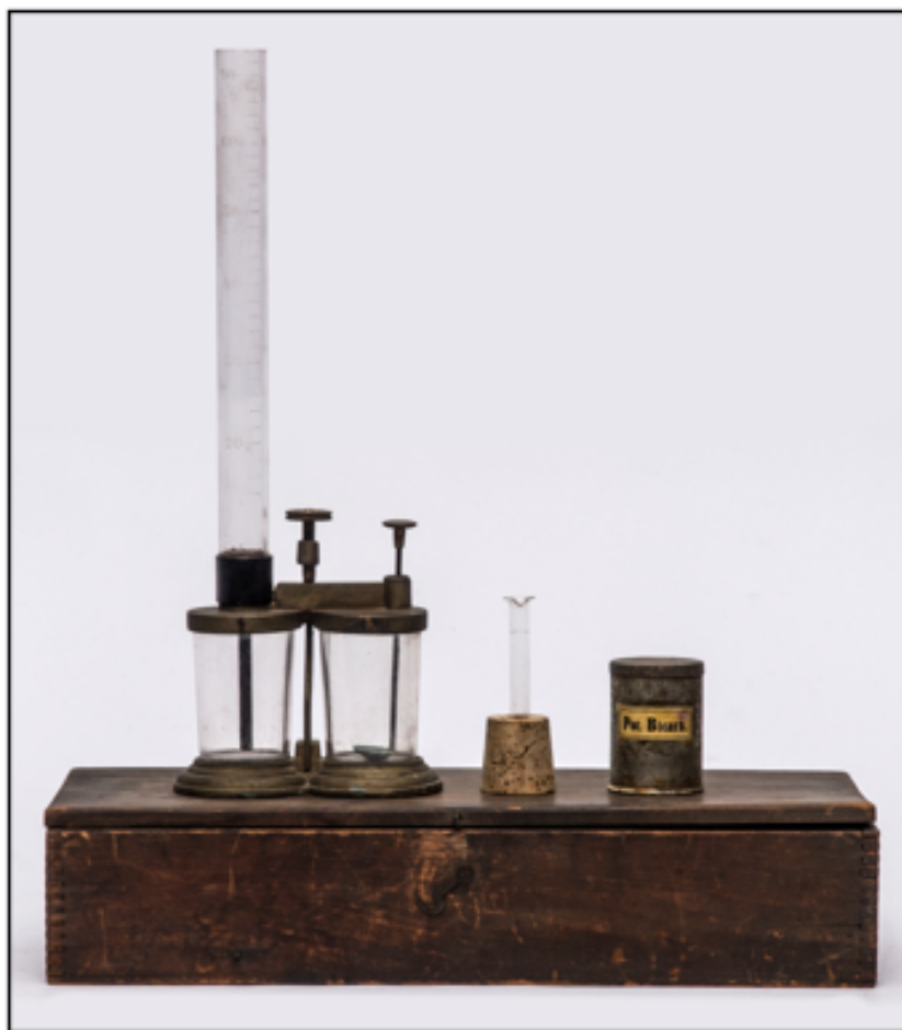
Figure 5. The Twitchell acidometer resting on top of its storage box. From left to right: the acidometer, the calibrated test tube for measuring out vinegar samples, and a small tin of potassium bicarbonate for charging the reaction spoon (Jensen-Thomas Apparatus Collection).
