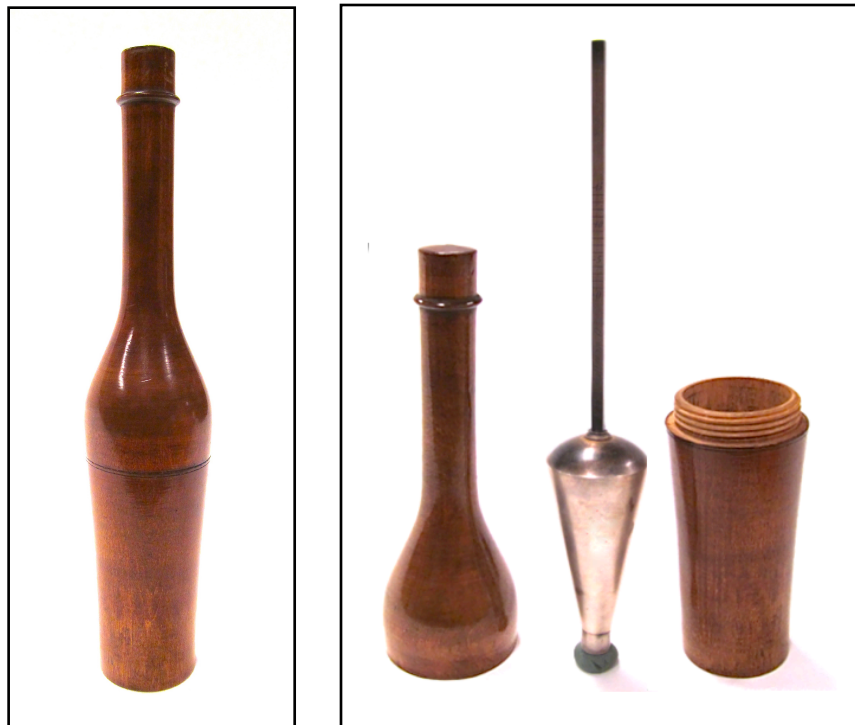
Figure 7. (Left): The closed (1.5" x 9") wine-bottle shaped maple case containing Twitchell's alcohol hydrometer. (Right): The case opened revealing Twitchell's (1.25" x 7.75") portable metal hydrometer for determining the alcohol content of wine and spirits.
