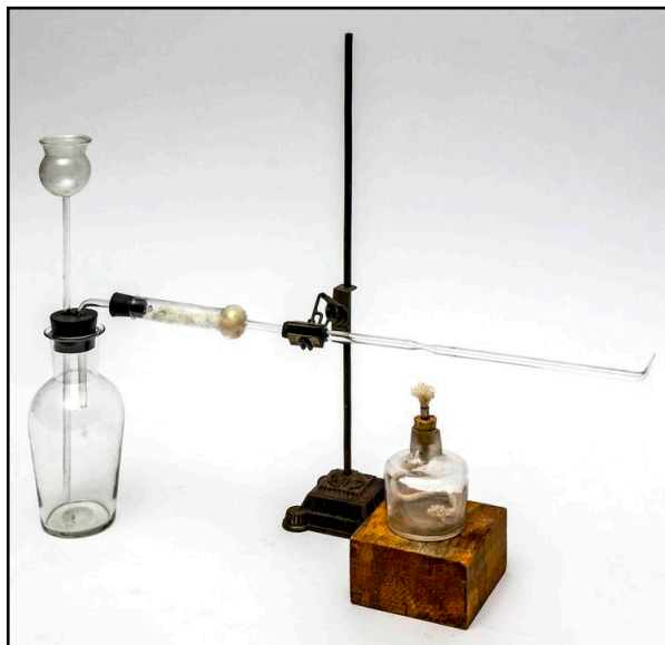
Figure 7. A reproduction of Berzelius' modification of the Marsh apparatus similar to that in figure 6 (Jensen-Thomas Apparatus Collection).
