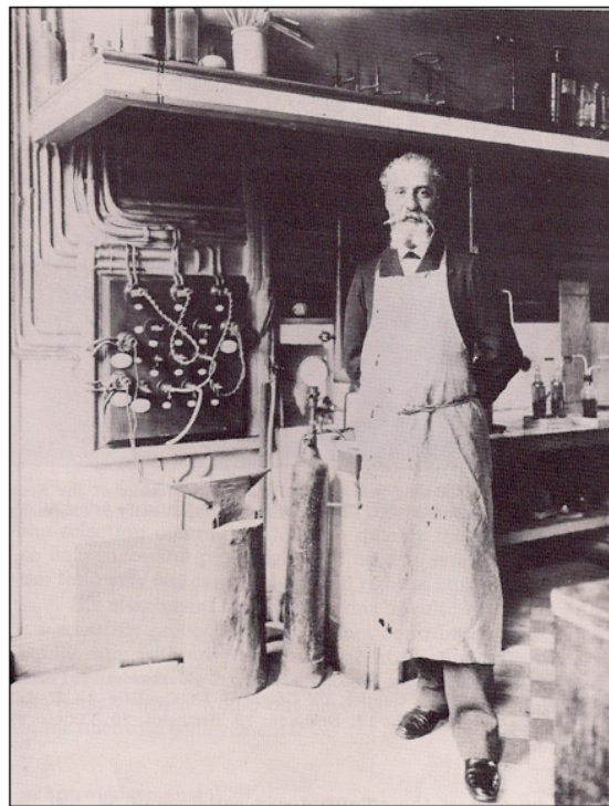
Figure 2. Ferdinand Frederik Henri Moissan (1852-1907) in his laboratory, c. 1895. Note the control board for his electric furnace and the anvil, presumably used in his diamond experiments.
