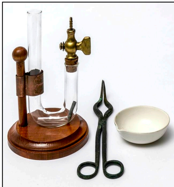
Figure 3. Reproduction of a Marsh apparatus similar to that in figure 2 (Jensen-Thomas Apparatus Collection). A short section of glass tubing is placed in the bend of the U-tube in order to keep the rod of Zn metal in the short arm.
