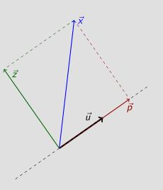
The orthogonal projection of  $\vec{x}$  onto  $\vec{u}$  is the pictured vector  $\vec{p}$  which is parallel to  $\vec{u}$  (so,  $\vec{p} = s\vec{u}$  for some scalar) and has the property that  $\vec{z} = \vec{x} - \vec{p} \perp \vec{u}$ .
