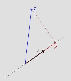
The orthogonal projection of  $\vec{x}$  onto  $\vec{u}$  is the pictured vector  $\vec{p}$
