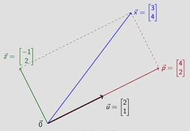
$$\vec{p} = \frac{\vec{x} \cdot \vec{u}}{\vec{u} \cdot \vec{u}} \vec{u} = \frac{10}{5} \vec{u} = 2\vec{u} \text{ and } \vec{z} = \vec{x} - \vec{p} = \begin{bmatrix} 3\\4 \end{bmatrix} - \begin{bmatrix} 4\\2 \end{bmatrix}$$
