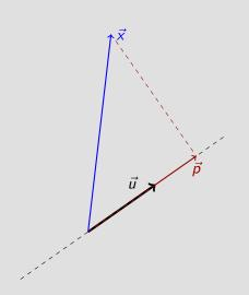
The orthogonal projection of  $\vec{x}$  onto  $\vec{u}$  is the pictured vector  $\vec{p}$  which is parallel to  $\vec{u}$  (so,  $\vec{p} = s\vec{u}$  for some scalar) and has the property that
