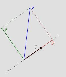
The orthogonal projection of  $\vec{x}$  onto  $\vec{u}$  is the pictured vector  $\vec{p}$  which is parallel to  $\vec{u}$  (so,  $\vec{p} = s\vec{u}$  for some scalar) and has the property that  $\vec{z} = \vec{x} - \vec{p} \perp \vec{u}$ . For this to hold, we need  $\vec{z} \cdot \vec{u} = 0$ , which allows us to determine s. We find that
